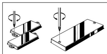
\* Instruments that have adjustable pole pieces can be adjusted to balance the output of each string.
